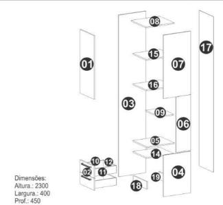
A Parafuso minifix (26x) 1416 K Puxador Livello (2x) 2118 B Tambor minifix (28x) 1417 L Parafuso minifix Duplo (1x) 1496 80 C Prego 11x11 (42x) 1669 M Suporte de prateleira (4X) 349 D Sapata (4x) 344 N Tapa Furo 19mm (16x) E Cavilha 6x30 (30x) 46 0 Tapa Furo 15mm (2x) C. S. F Dobradiça 35mm (2x) 1987 Р Cola 5g (1X) 13 Parafuso cab. Chata 3,5x14mm (26x) Parafuso Flang G hans 132 Q Adesivo (1x) 225 H Parafuso Flang
